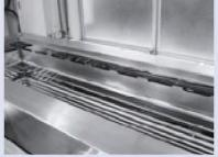
Increasing volume of cooling coil in order to raise free board ratio
