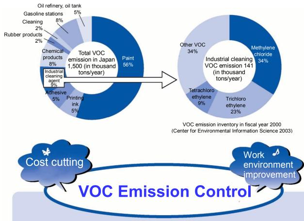
VOC emission control measures in industrial cleaning are generally organized in the "VOC emission control organization chart" (P.1). While introducing retrieval/recycling equipment of cleaning agent vapor is an effective measure, low-cost technology measures for improvement of cleaning process (improvement of operation, modification of cleaning equipment) are also effective as well as being simple.
