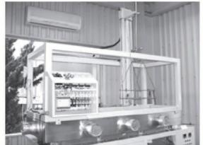
Transport equipment with model cleaning equipment for quantitative measurement experiment (Source: Industrial Cleaning VOC Manual Committee WG)
