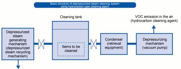
Emitting cleaning agent waste liquid with processing oil mixed in (processing oil + hydrocarbon type cleaning agent)
